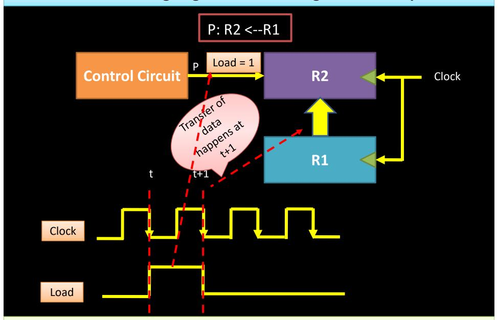
Note that the clock is not included as a variable in the register transfer statements. It is assumed that all transfers occur during a clock edge transition.
